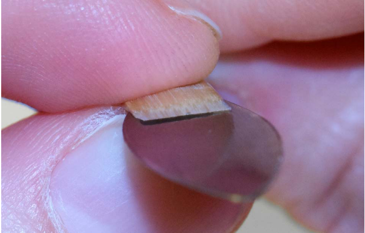
Figure 20: Photograph, a reed failing the plaque test. Photo by Dylan Farnsworth
