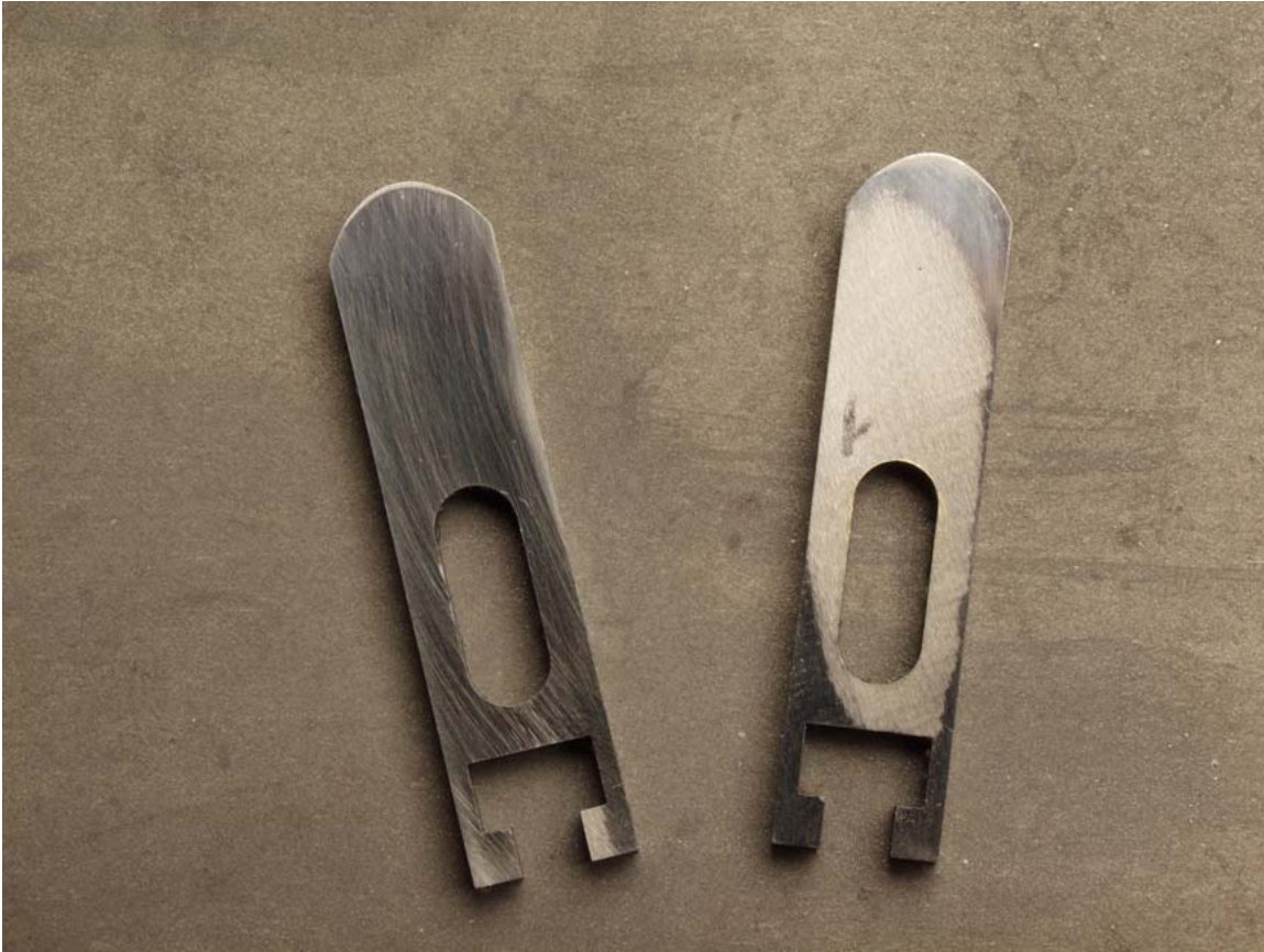
Figure 8: Photograph, worn blades. Photo by John Ferrillo
