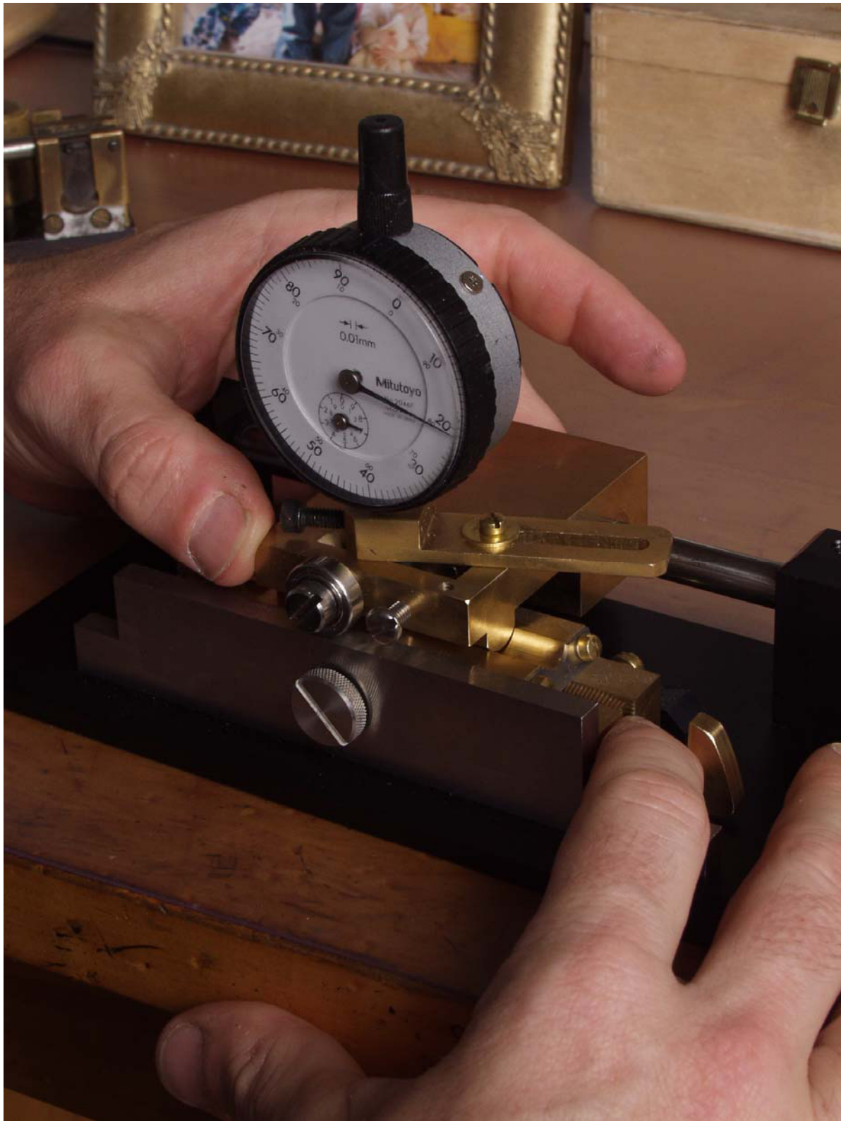
Figure 11: Photograph, an alignment jig on a machine. Photo by John Ferrillo
