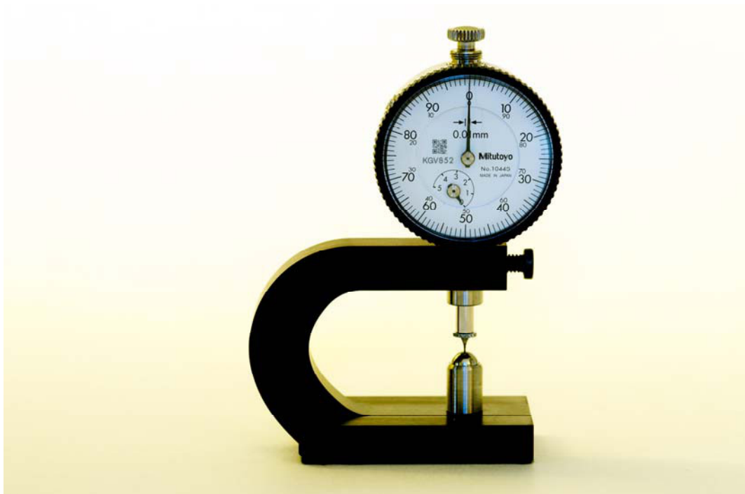
Figure 13: Photograph, the HDR dial indicator. Photo by Dylan Farnsworth
