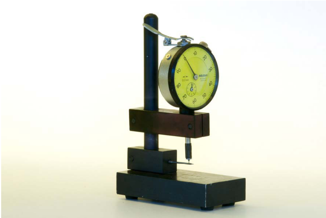
Figure 14: Photograph, a dial indicator with a replaced tip. Photo by Dylan Farnsworth
